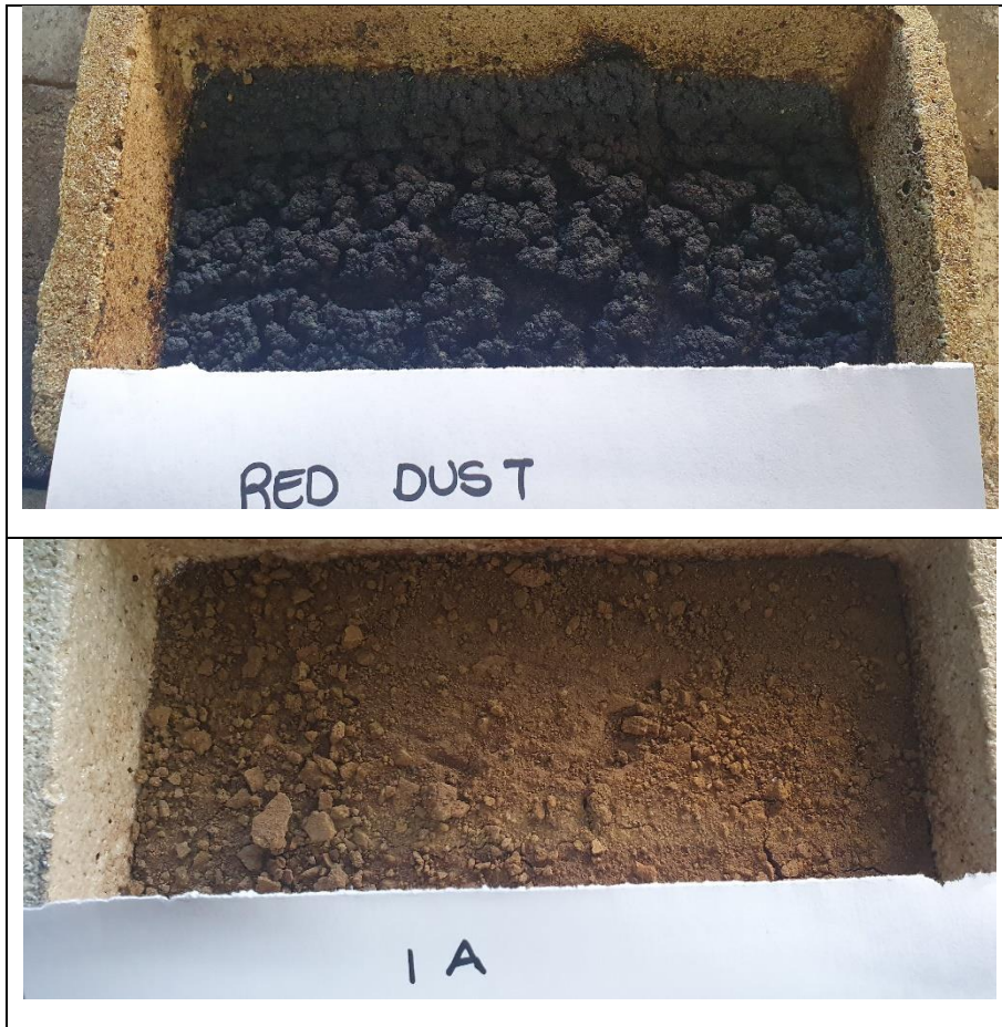
Figure 4 Appearance of the red dust and 1A samples after roasting at 1100°C
