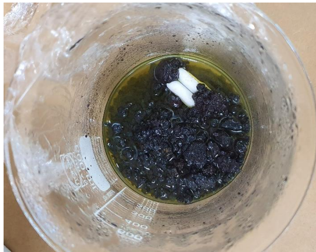
Figure 6 Appearance of the leach slurry of the un-milled roasted red dust sample at 1000°C
